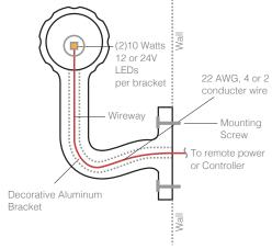
EpicRail™ is an LED-based illuminated handrail. This energy efficient, color changing and programmable sustainable solution addresses the architectural need for a handrail that produces safety required illumination levels for both interior and exterior stairs, ramps and walkways.
